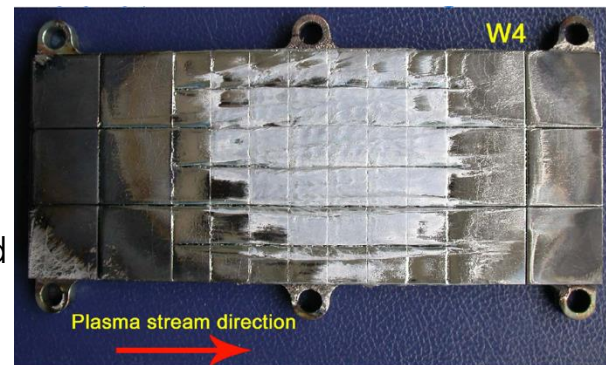
Russian ELM simulator, showing damage to Tungsten surface with ITER ELM-like plasma bombardment
