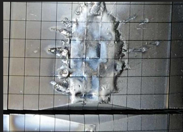
JET runaway electrons damage. https://www.iter.org/newsline/-/2234
