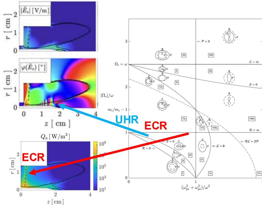
Studies show that parametric bounding surfaces affecting wave propagation in cold plasmas suffice to explain the thruster heating mechanism.
