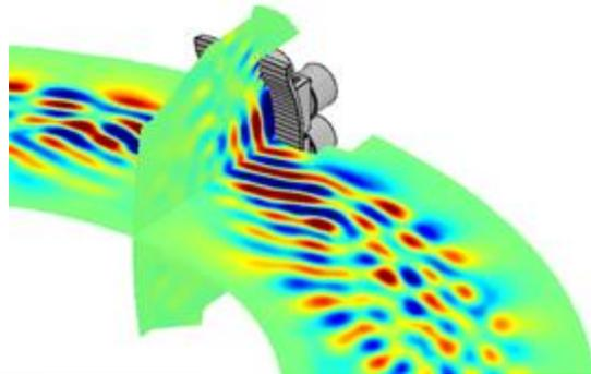
Mode conversion to a backward mode called the ion Bernstein wave (IBW). FW can still exist after the IIH. IBW absorbed by electrons via Landau damping. Conversion sensitive to minority concentration.
