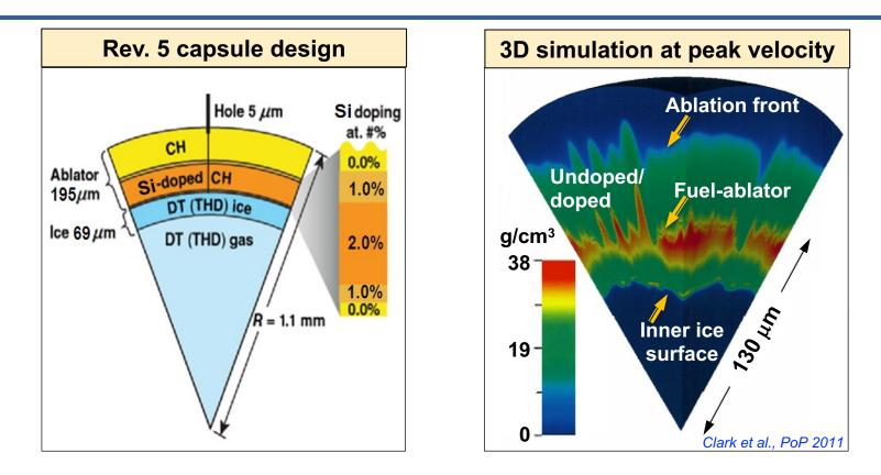
Mixing of ablator material into the hot spot due to the hydrodynamic instabilities can increase the radiative cooling and degrade capsule performance in ICF implosions
