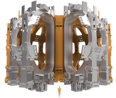
ITER Toroidal Magnetic Field Coils
