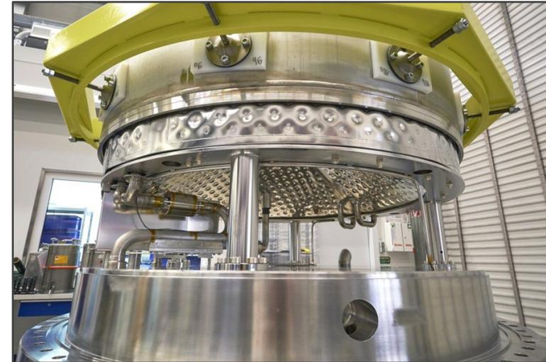
**Figure 2.** Photograph of ITER cryopump. *Source: ITER.org.*
