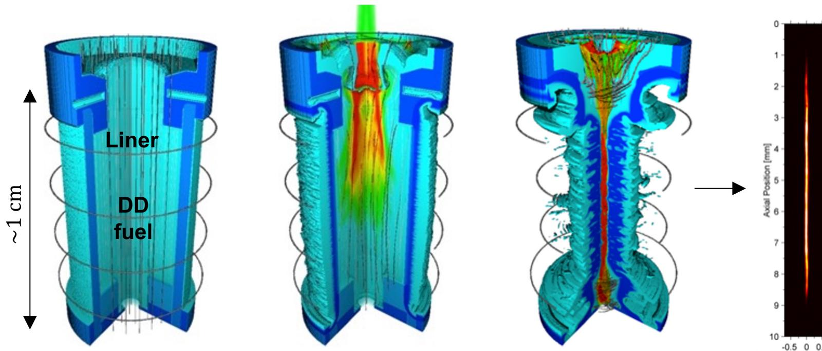
Fuel is premagnetized with an axial B-field, reducing conduction losses and trapping alpha-particles
