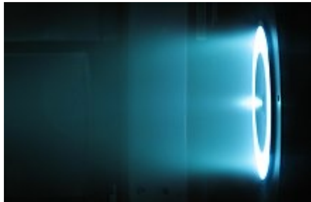
6 kW Hall thruster in operation at the NASA Jet Propulsion Laboratory
