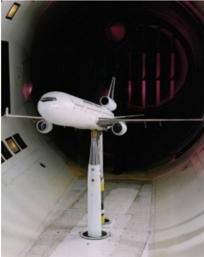
*Wind tunnel experiments use dimensionless scaling*
