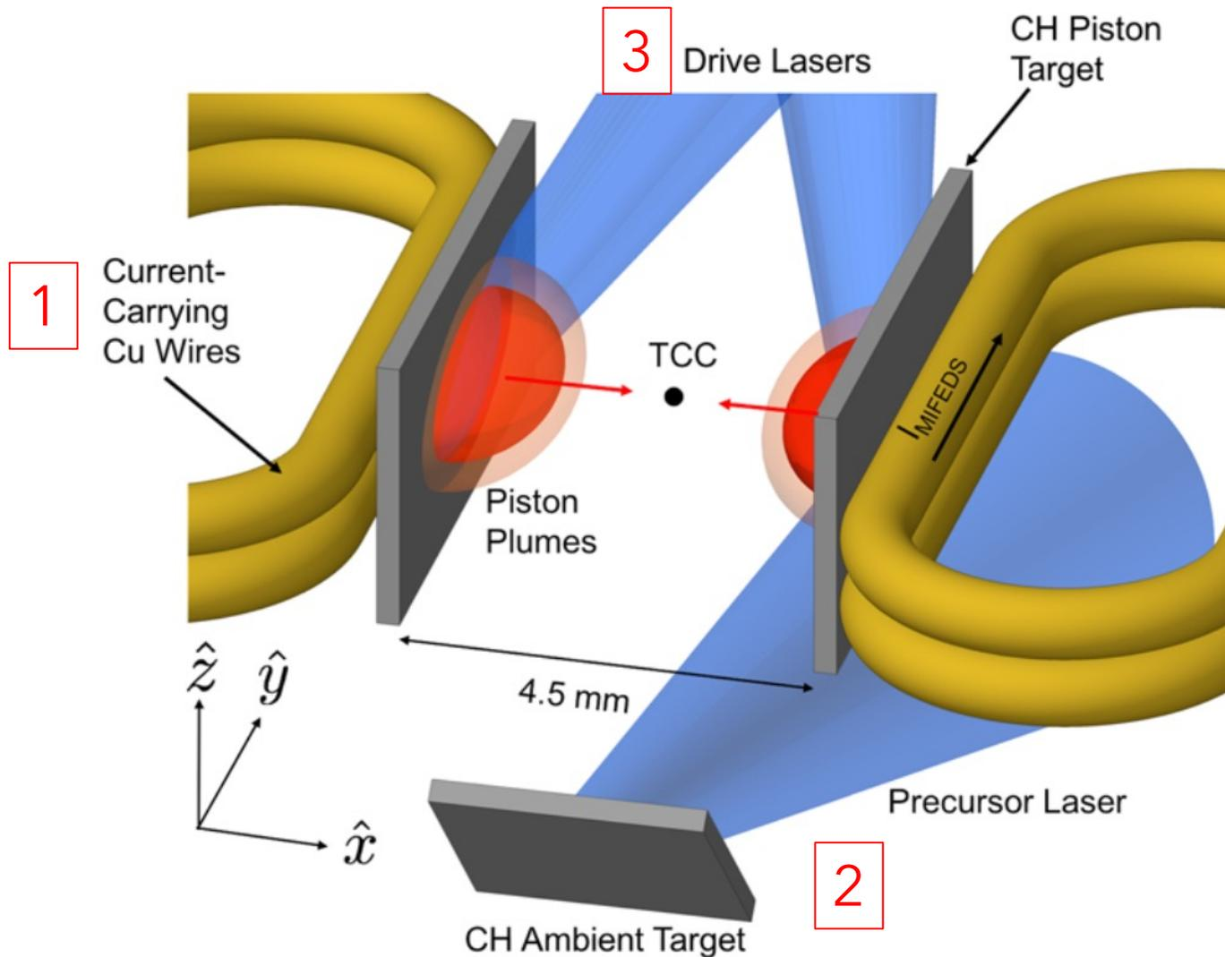
1. Magnetic coils fill volume with  $B_z = 8$  T field
