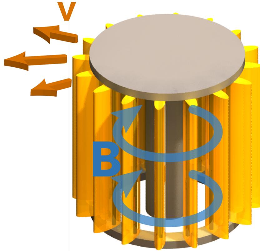
Current **heats** the wires & generates the **magnetic field** which **accelerates** the plasma
