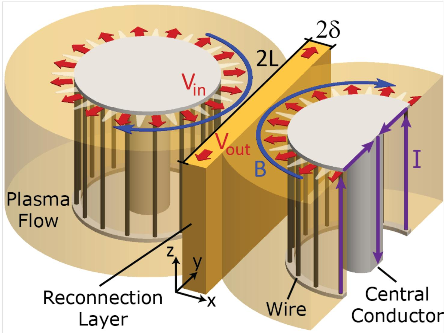
Drive two exploding arrays in **parallel**: collides flows with **opposite magnetic fields**, forming a **reconnection layer**.
