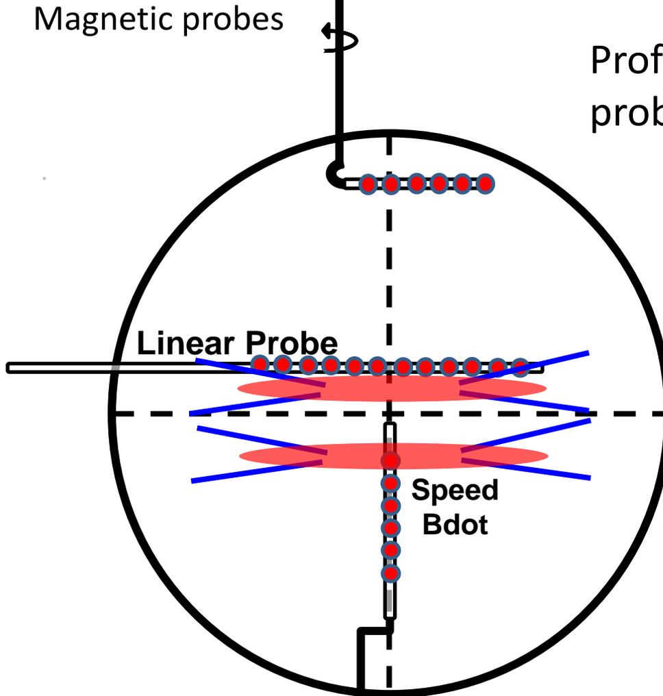
Profiles can be built from movable probe, using multiple shots
