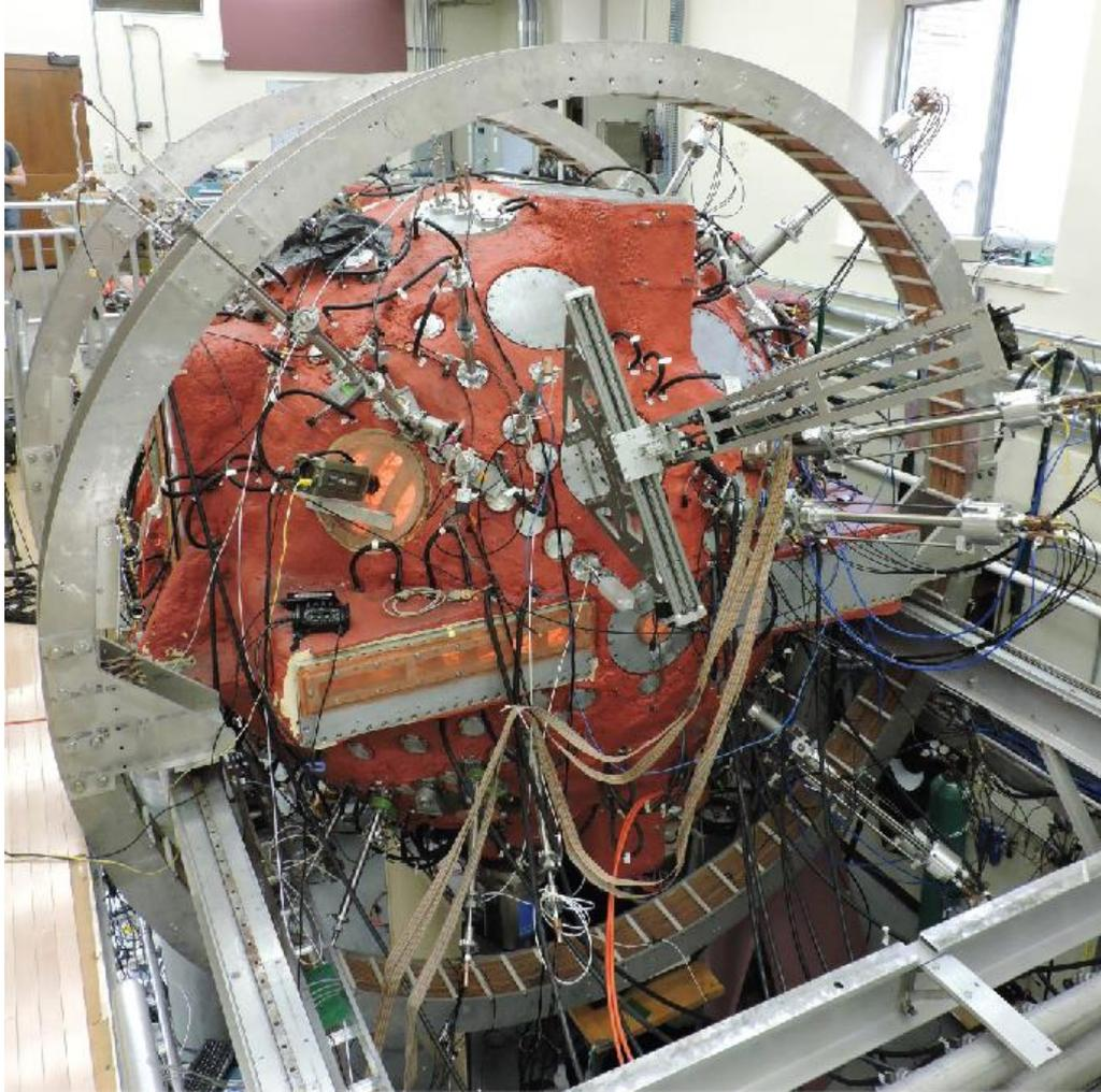
The BRB (Big Red Ball) is comprised of a 3m diameter vacuum vessel.
