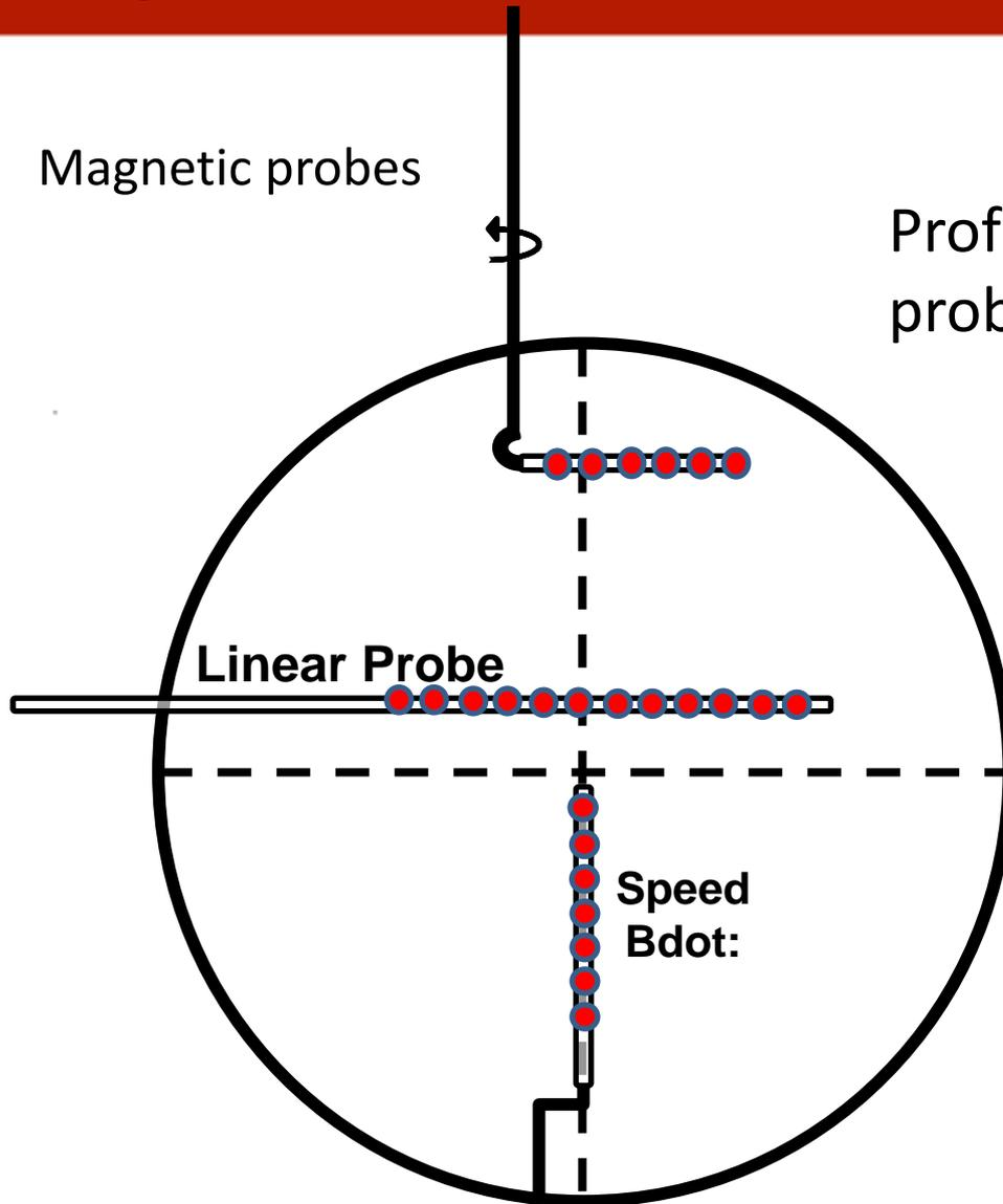
Profiles can be built from movable probe, using multiple shots
