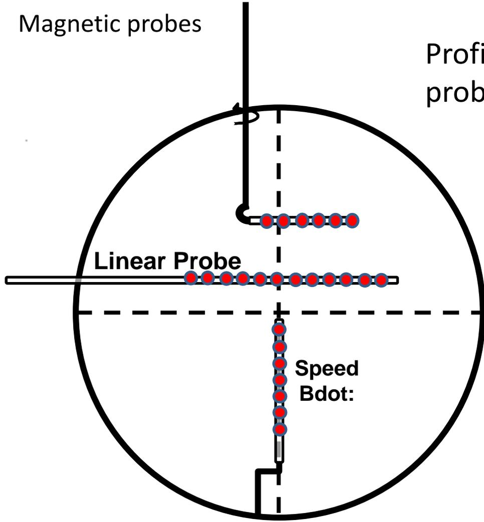
Profiles can be built from movable probe, using multiple shots
