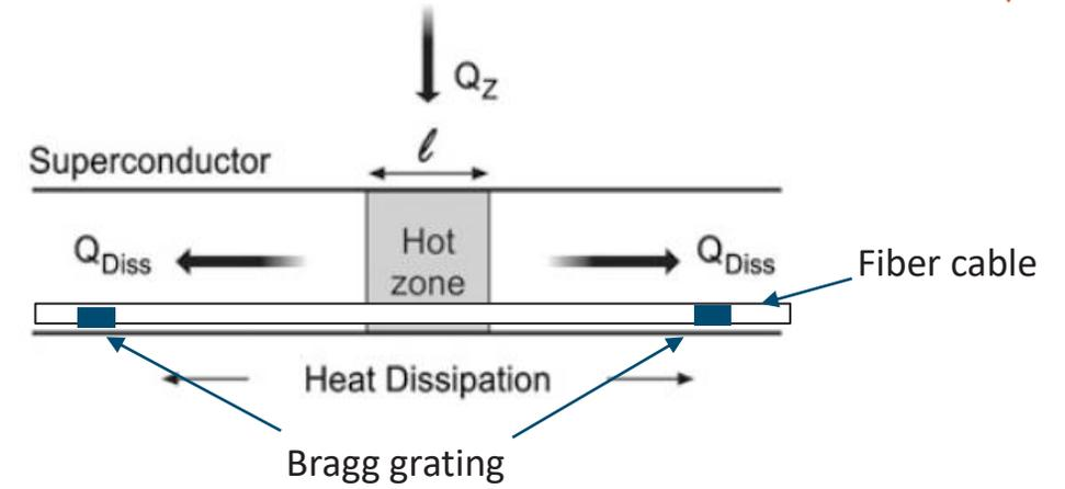
Working principle of fiber Bragg grating technology
