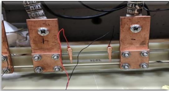
HTS tape Ic characterization test setup
