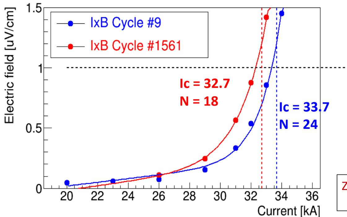
Bravo Cycles : 5K, 10.9T, 35kA ( $382 \text{ kN/m}$ )
