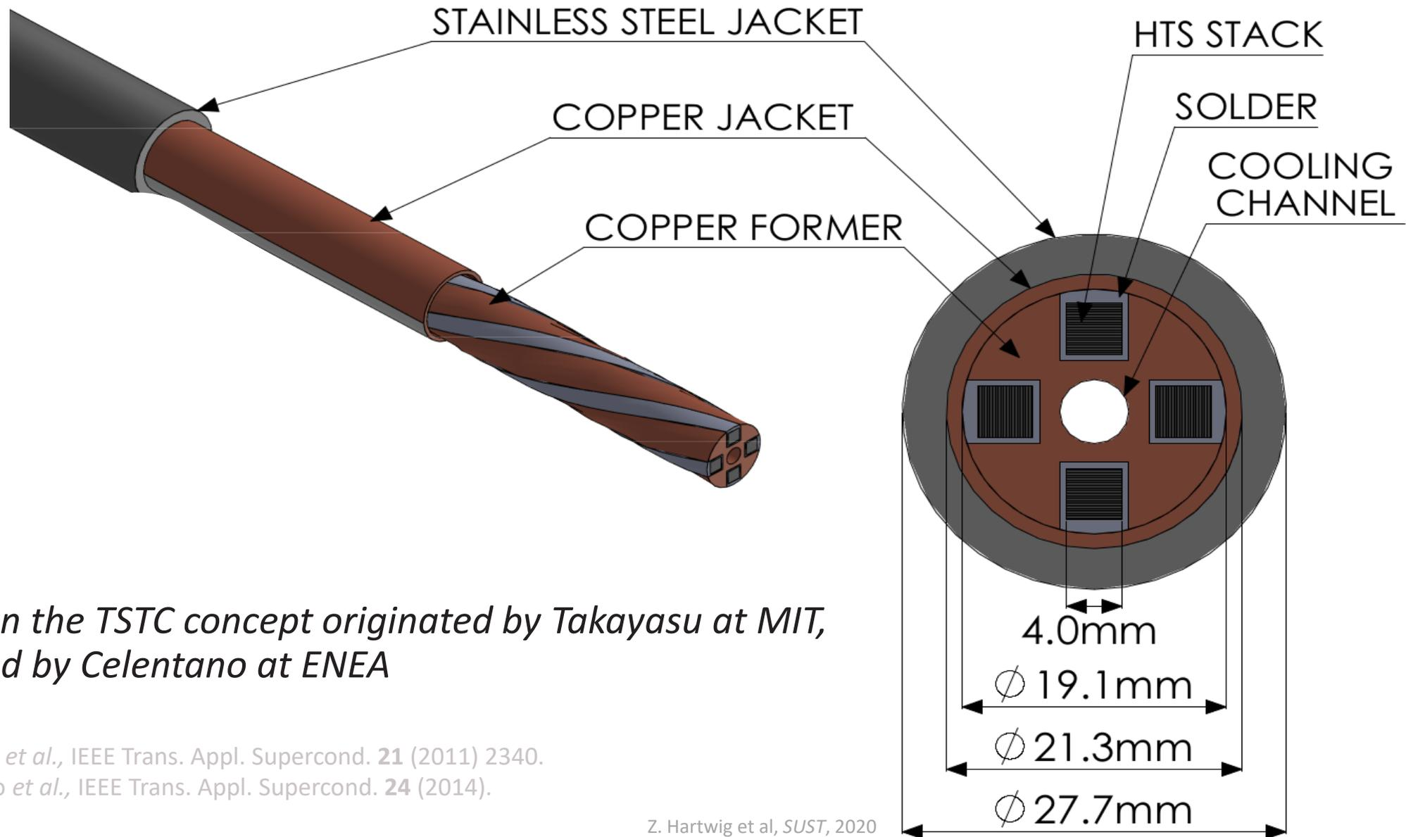
*Based on the TSTC concept originated by Takayasu at MIT, extended by Celantano at ENEA*
