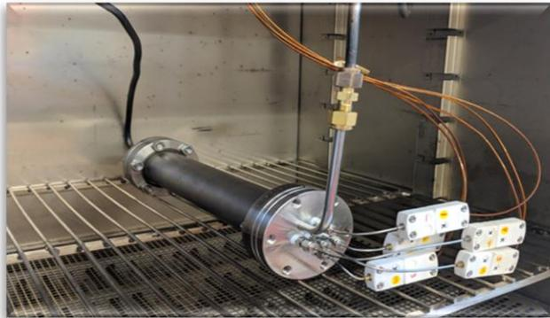
HTS tape oven test rig
