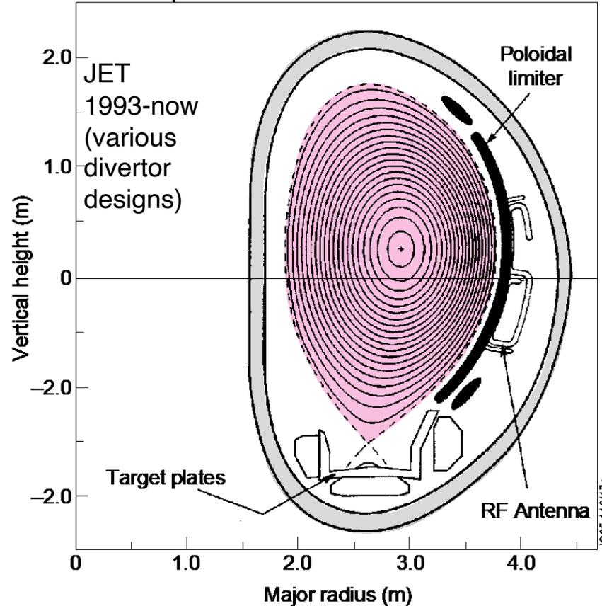
If external current is run in the same direction as plasma current *outside* of the confined plasma, then one component of the field can be canceled, creating an **X-point divertor**
