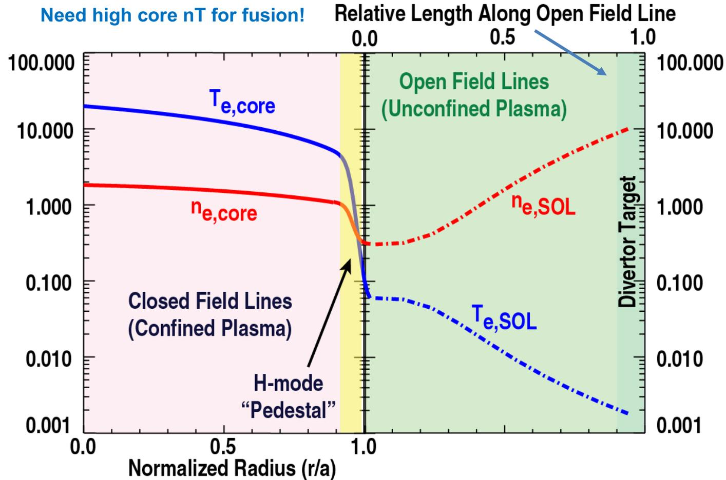
**H-mode pedestal:** mediates the tension between the core and the edge and influences the performance of both
