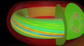
Nonlinear simulation of Toroidal Alfvén Eigenmode (TAE) evolution performed with MEGA code (courtesy Y. Totsu)
