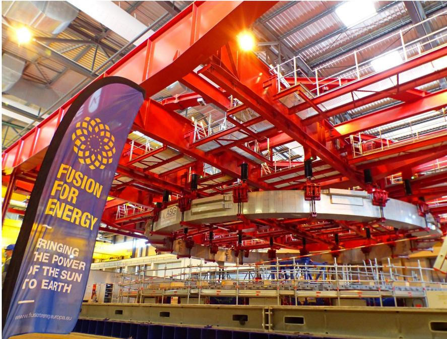
Poloidal Field Coil #5 nearing completion, April 2020
