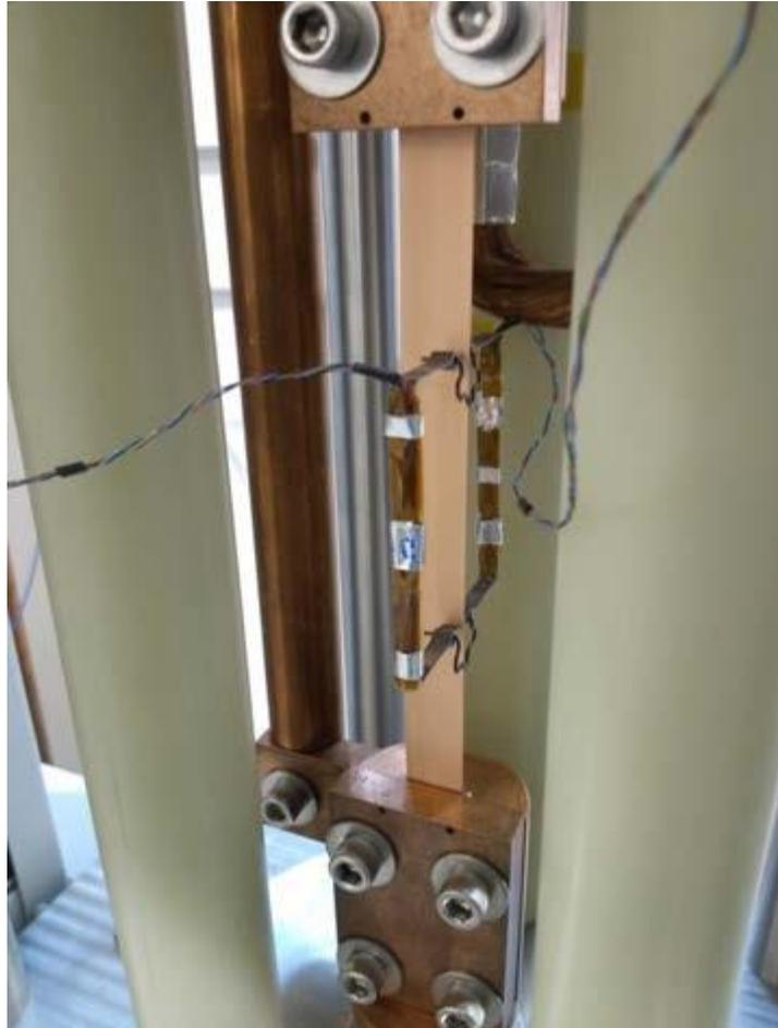
Cryogenic, axial tensile test station
