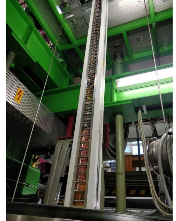
*SPARC SULTAN EM loading samples being instrumented and installed*
