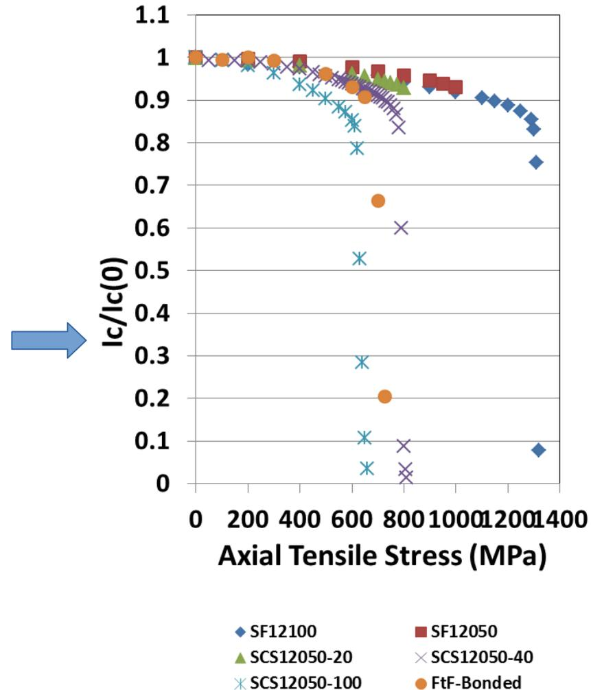
5% critical current degradation occurs at 600-800 MPa and ~0.45% strain for most tape formulations
