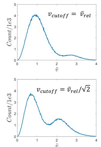
Figure 5: Speed distribution after cooling for 10 sound times using two different values for the cutoff relative velocity. No compression or potential was used.
