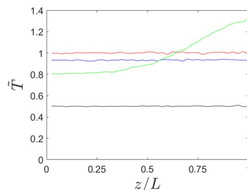
Figure 3: Temperature profile for fast compression using coulomb collisions. Black: initial profile; red: upon heating; green: at maximum temperature gradient; blue: at new equilibrium.  $G = 2.5$ ,  $\delta = 1$
