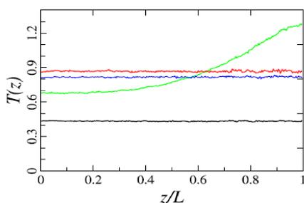
Figure 2: Temperature profile for fast compression from Geyko. Black: initial profile; red: upon heating; green: at maximum temperature gradient; blue: at new equilibrium [1].
