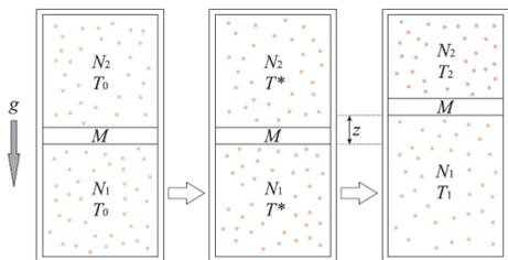
Figure 1: Description of piezo-thermal effect for gas heated from  $T_0$  to  $T^*$  separated by a partition of mass  $M$  [1].
