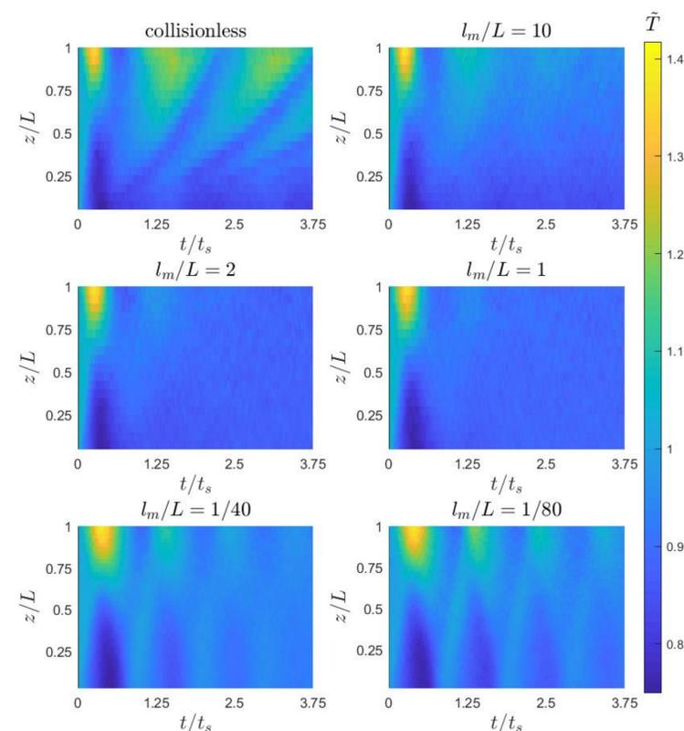
Figure 4: Temperature profiles over time for several values of  $l_m/L$ . Time variable has been normalized to the sound time ( $t_s$ ).  $G = 2.5$ ,  $\delta = 1$
