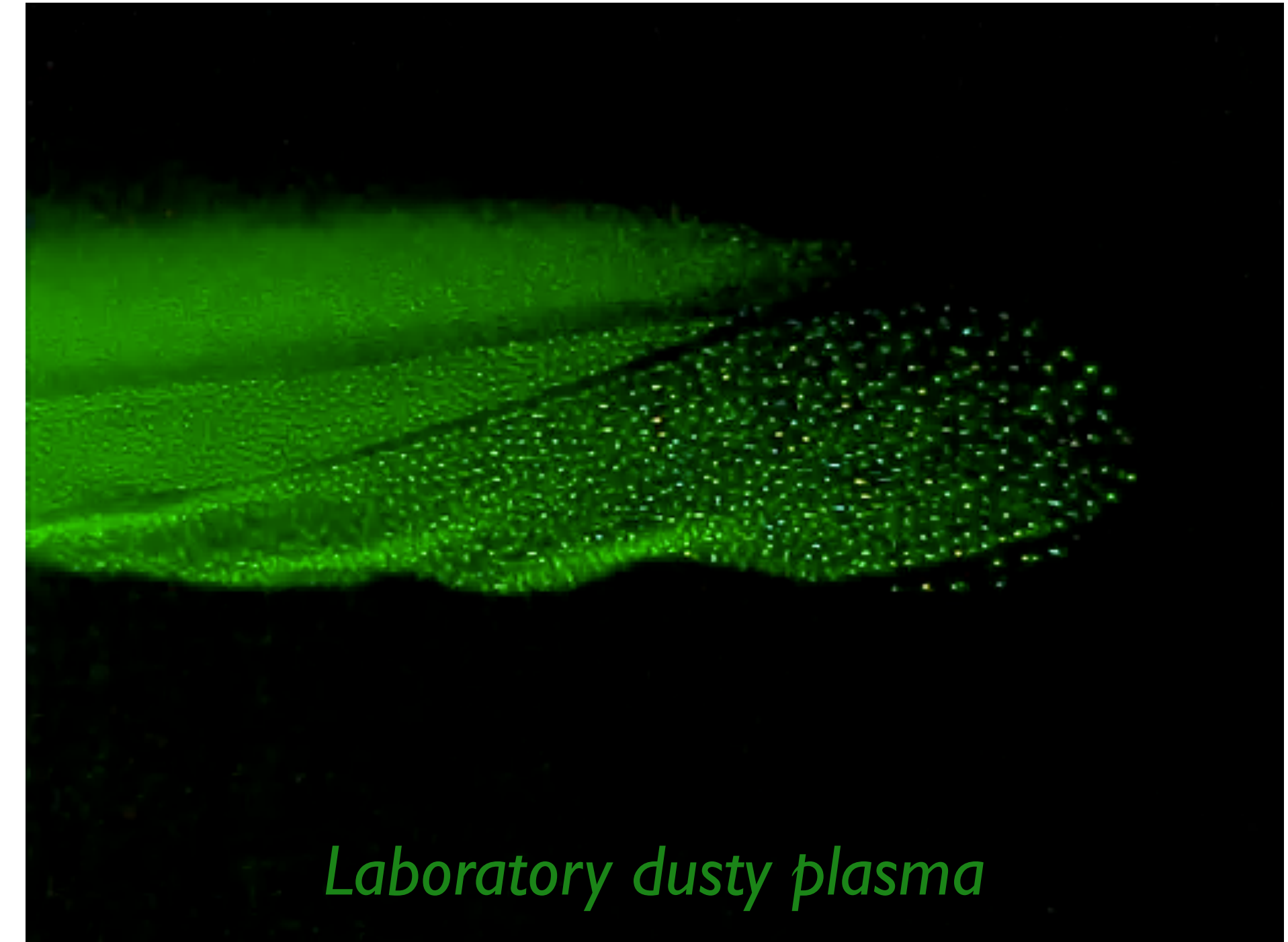
Laboratory dusty plasma 3-micron silica particles in an argon plasma (1/10th speed) [Auburn University]
