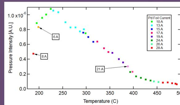
Graph showing the inverse temperature vs permeation rate of the data taken when the nichrome wire heater was cooled down from 500°C
