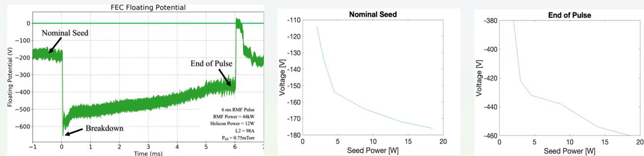
Assuming  $T_e > T_i$  and a Maxwellian distribution, the Floating Potential can be converted to an equivalent electron energy.
