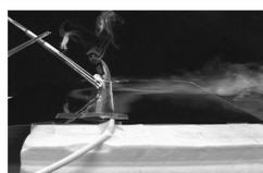
Fig. 1 Electrically safe non-thermal  $\alpha$ -plasma for treatment of living tissue without causing damage
