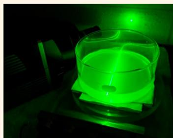
Figure 4: LAS setup. The laser is shot through the center of the glass container, with the PI camera capturing the image on WinSpec software.
