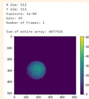
Figure 3: Image of laser as shown on Python. The exposure of the camera could be adjusted to better capture the pixels and their associated brightness.
