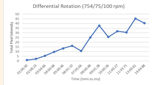
Figure 5: A plot of AACC's intensity over time during differential rotation. Fourteen samples were taken every 60-seconds, for about 14 minutes.
