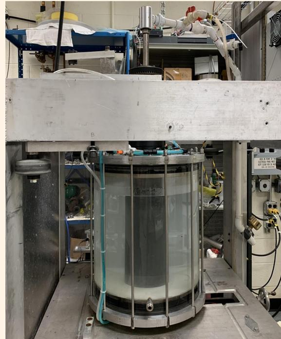
Figure 2 AACC. The black cylinder represents the inner cylinder while the clear cylinder is the outer cylinder. The network of inlets and outlets can be seen by the series of blue and clear plastic tubes lining the sides and top of the apparatus. The deposit and recycling bucket (not shown) are to either side.
