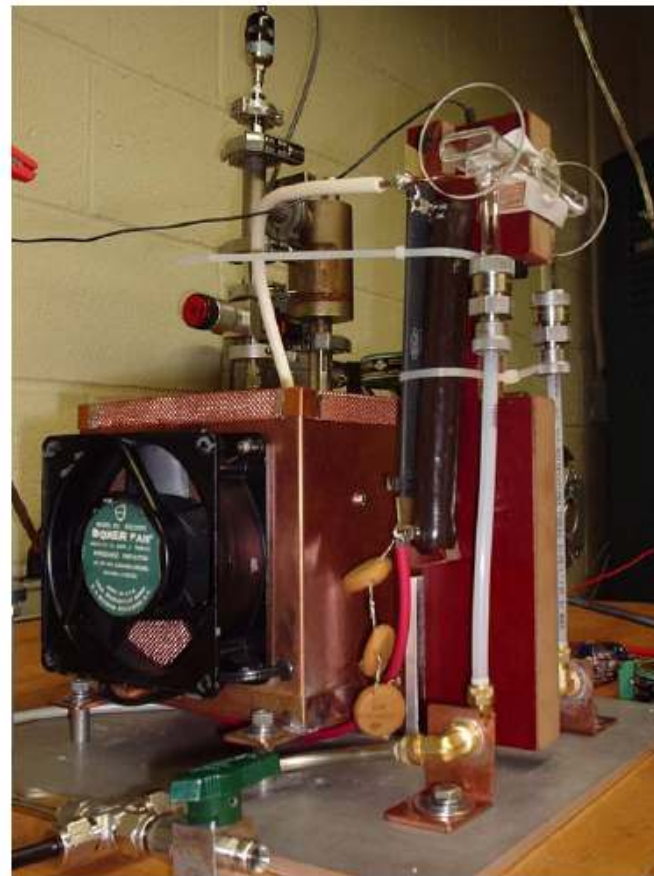
Side view of the DBD cell experiment with the fast high voltage transistor switch connected to the bottom electrode.
