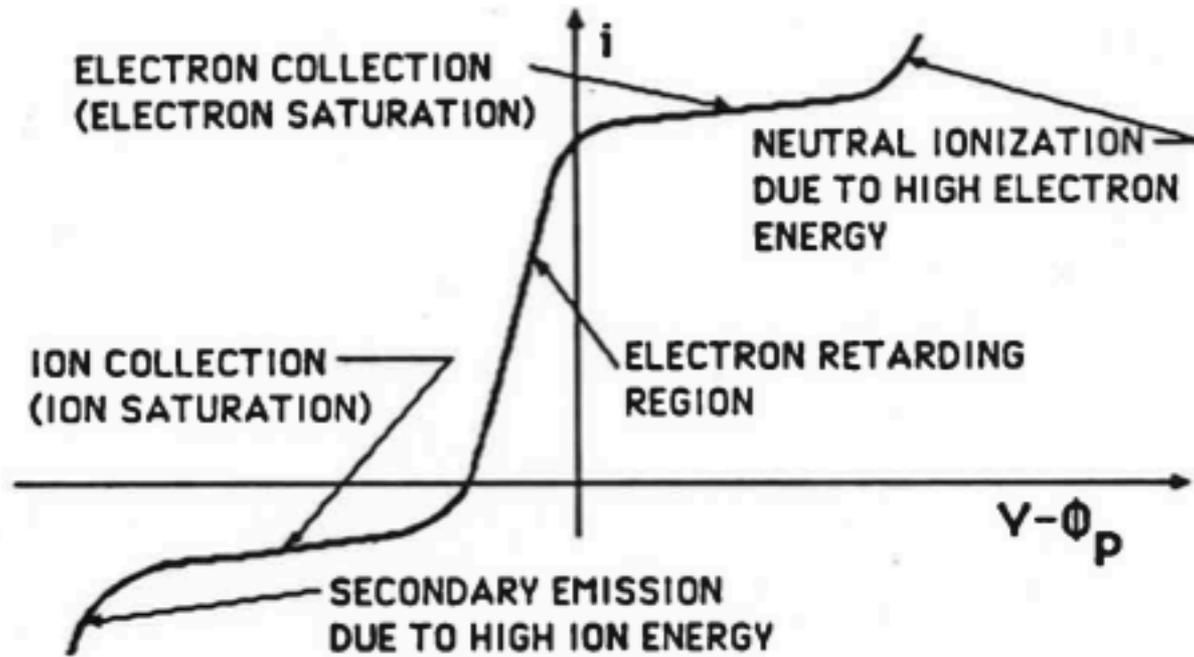
Figure 2: Typical probe characteristic
