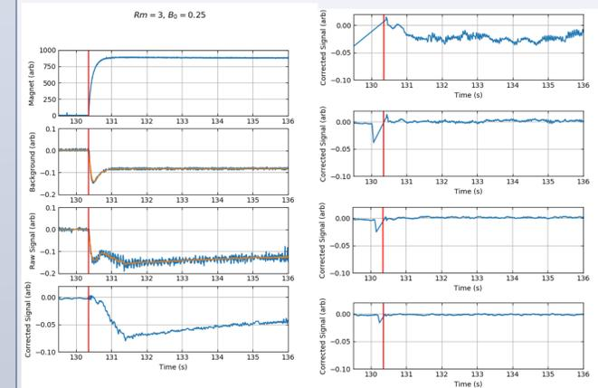
This data was collected from the top Hall sensor under the same conditions as the bottom Hall probes. They display the similar MRI signals as the bottom Hall probes.
