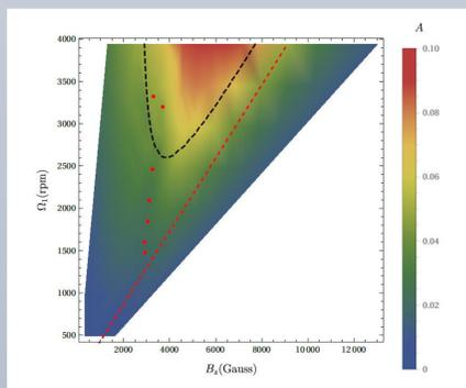
Numerical simulation results by Himawan Winarto [2]. Black dotted line indicates MRI unstable region predicted by simple linear model. Red dots indicate non-linear magnetic field signal in simulations indicating MRI instability.
