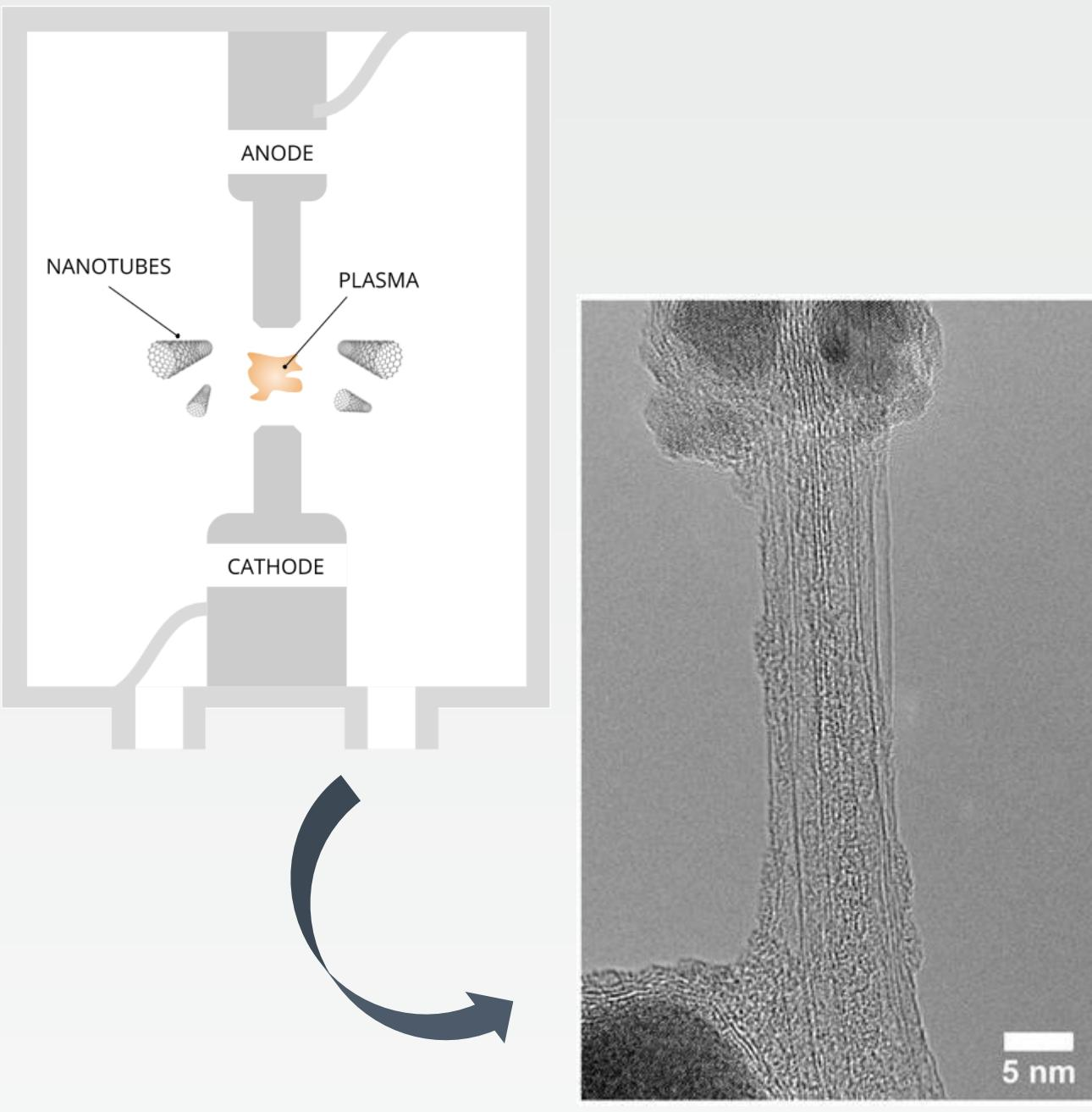
**Figure 2.** (left) The plasma arc synthesis method consists of the following: an inert gas environment, the anode which holds the material to be ablated, and the cathode on which the nanostructures are formed. **Figure 3.** (right) Example of a single-walled BNNT cluster formed in
