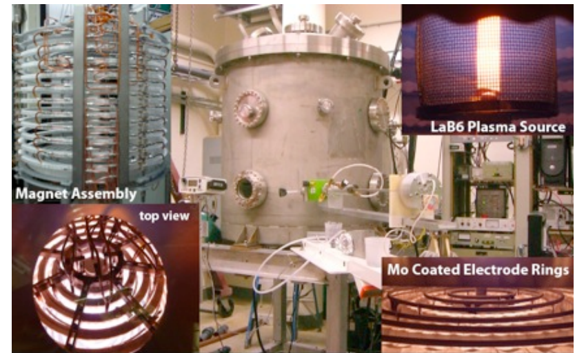
Plasma Couette-flow Experiment
