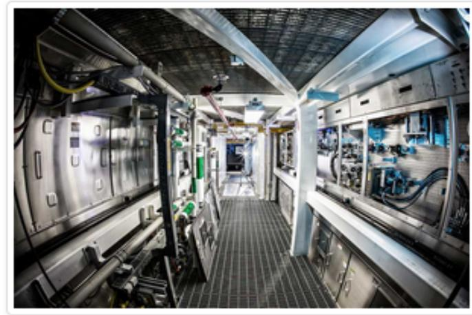
From the main amplifier, the beam makes a final pass through the power amplifier. By now, the beams’ total energy has grown from 1 billionth of a joule to 4 million joules—all in a few millionths of a second.
