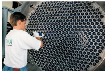
Ozone generation for water cleaning
