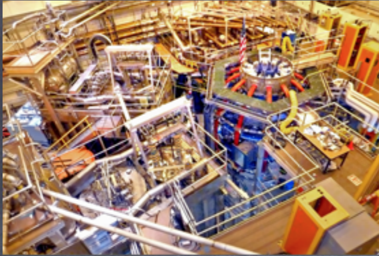
USA, San Diego: DIII-D medium-size tokamak
