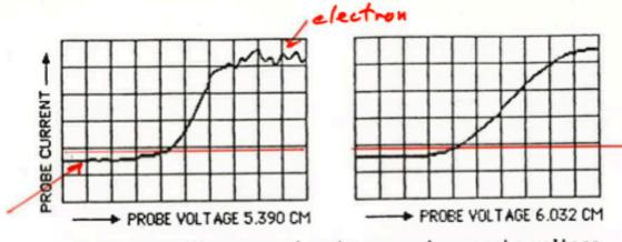
Typical oscillograms of probe current vs. probe voltage for different probe positions taken at 7, +1600 µsec
