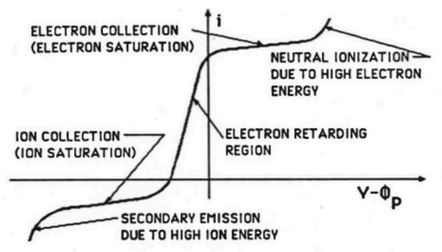
Figure 2: Typical probe characteristic
