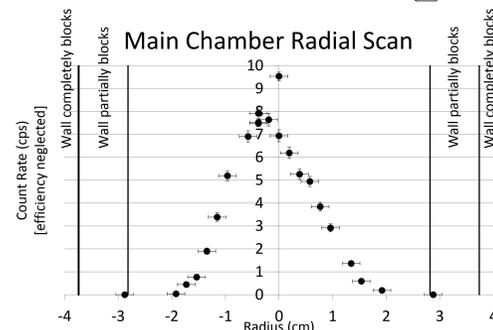
A scan across the radius of the plasma from the main chamber. That there is a sharp peak and not a flat rectangle (well within where the walls are expected to interfere) indicates X-rays originate from the core of the plasma rather than the surface.
