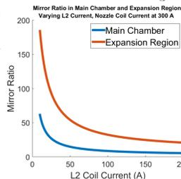
Instead, the observed increasing count rate may be explained by the small opening in the nozzle coils: the decreasing mirror ratio expands the field lines, leading to wider particle trajectories and causing particles to spiral into the wall.
