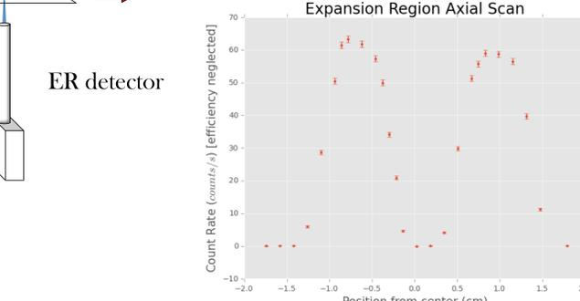
A scan across the axis of the plasma in the expansion region. Because the detector is partially blocked by a flux conserver (slightly to the right of zero), there is a valley in the middle of the two peaks where the count rate decays to zero.
