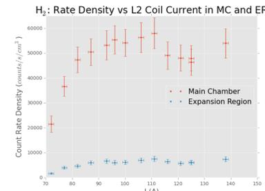
In the above, L2 current was varied with the ER and MC detectors recording X-rays simultaneously. To compare the count rates, the total count rates were converted to rate densities, showing a far greater source of X-rays in the MC. This could be due to mirror effects or the plasma radius.
