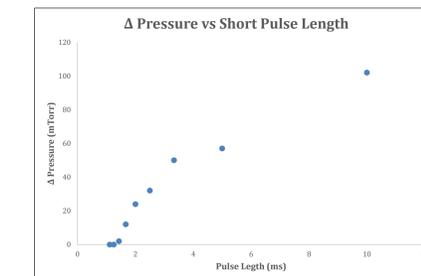
In the short pulse regime (to the left) the change in pressure goes roughly linear until the duration falls below 2ms at which point the change rapidly goes to zero. This is because the valve fails to open. The reason for this is most likely that the amount of electrical energy applied is insufficient to produce the impulse necessary to move the crystal any faster.
