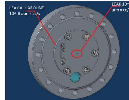
The "sealing force" of the crystal was found using the pressure differential. The vacuum applies no pressure so the atmosphere applies the only force equal to:  $F = P\pi r^2 \approx 10^5 \pi (0.0025)^2 \approx .02N$  which is about 5% of the maximum load force of the crystal.
