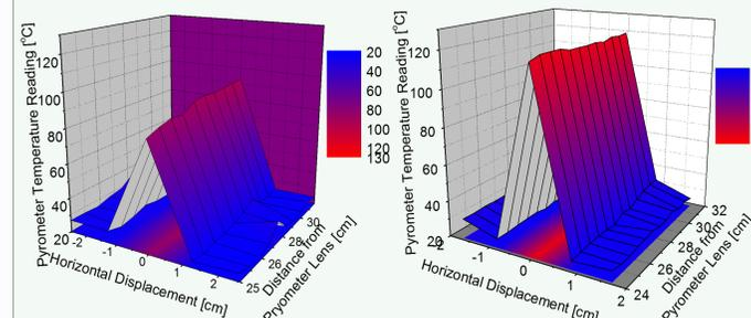
Projected areas of sample holder at 30° and 60° on pyrometer field of view
