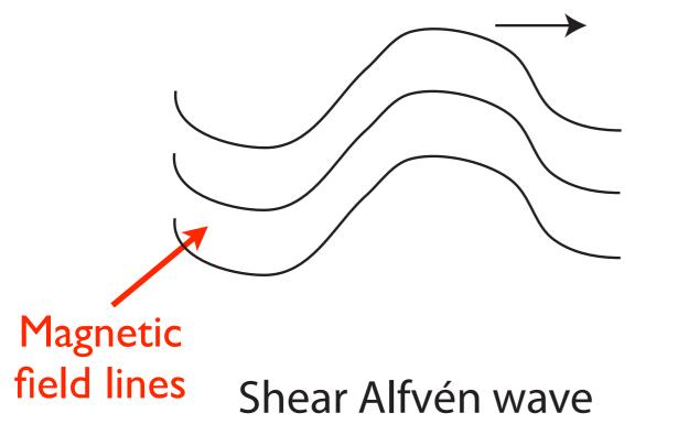
Shear Alfvén wave: analogous to wave on string, tension provided by field line, mass by plasma
