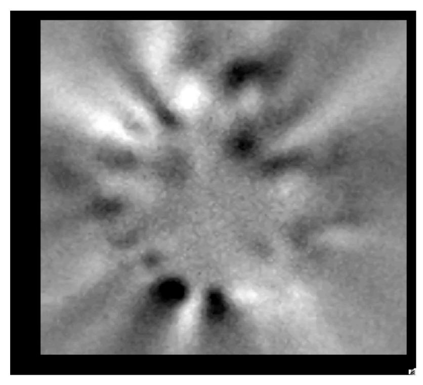
Fast framing camera (~50k frames per second, ~10ms total time), visible light (neutral He), viewed along B
