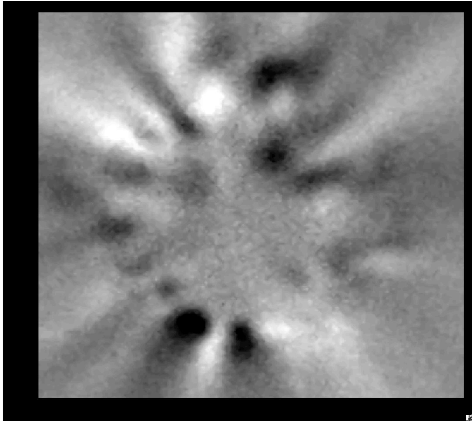
Fast framing camera ( $\sim 50\text{k}$  frames per second,  $\sim 10\text{ms}$  total time), visible light (neutral He), viewed along B
