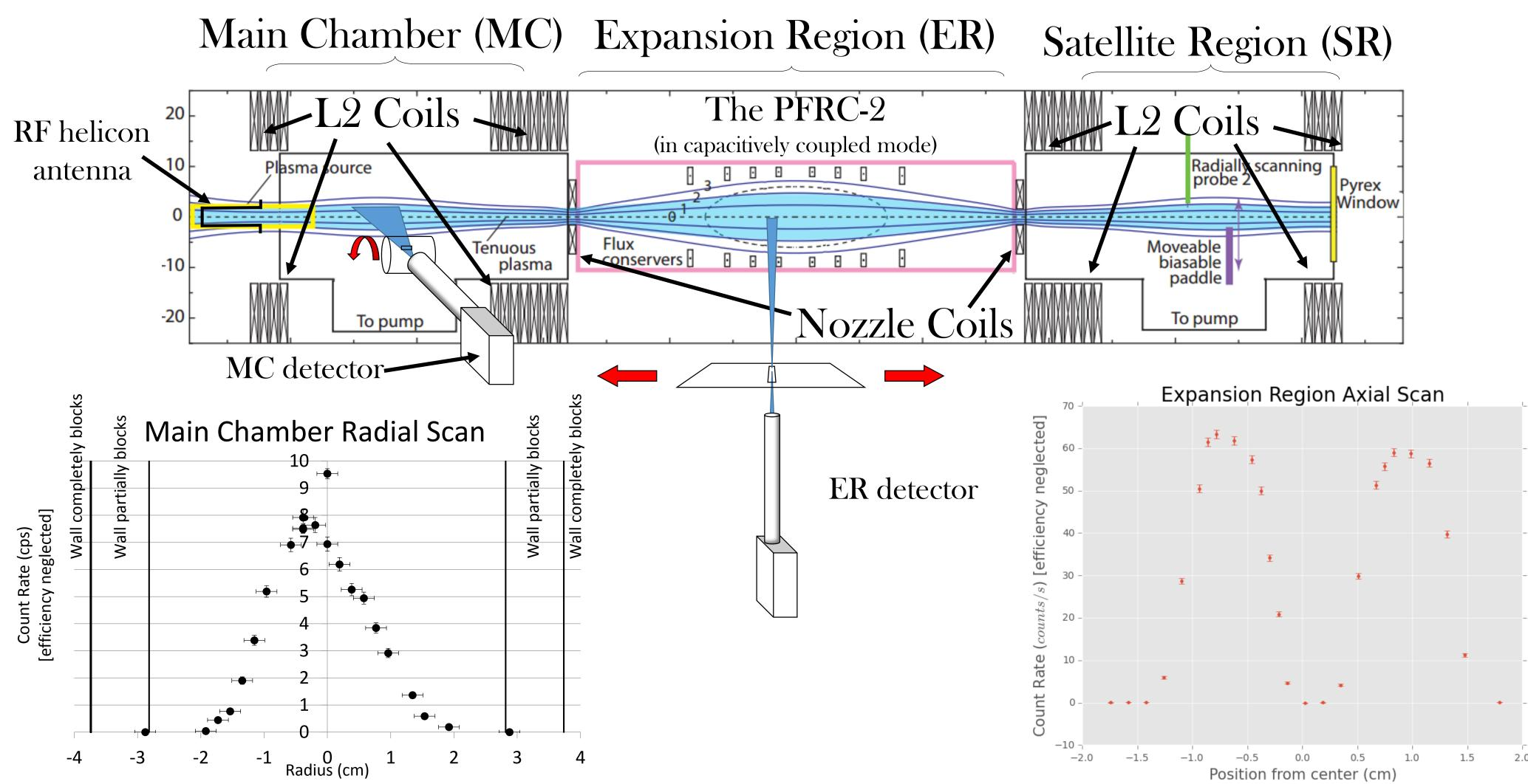
A scan across the radius of the plasma from the main chamber. That there is a sharp A scan across the axis of the plasma in the expansion region. Because the detector is partially blocked by a flux conserver (slightly to the right of zero), there is a valley peak and not a flat rectangle (well within where the walls are expected to interfere) in the middle of the two peaks where the count rate decays to zero. indicates X-rays originate from the core of the plasma rather than the surface.
