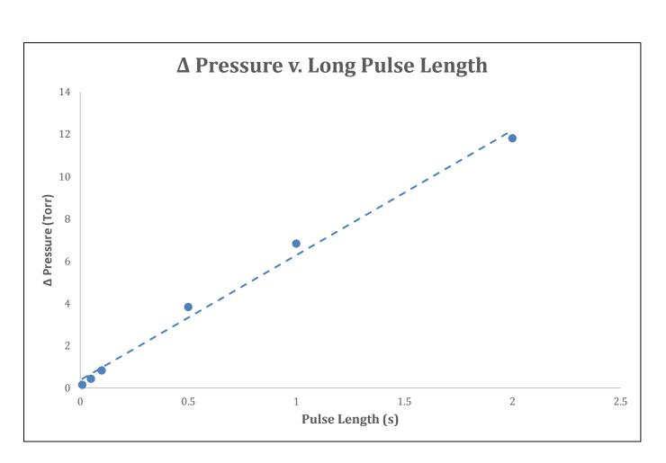
In the short pulse regime (to the left) the change in pressure goes roughly linear until the duration falls below 2ms at which point the change rapidly goes to zero. This is because the valve fails to open. The reason for this is most likely that the amount of electrical energy applied is insufficient to produce the impulse necessary to move the crystal any faster.
